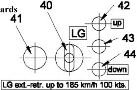
40) Toggle switch for extension and retraction of the electrically operated main landing gear
